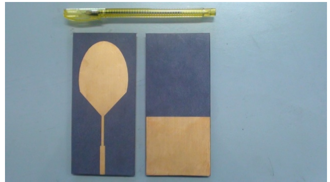
Figure 1 UWB Antenna front and back side
